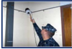
Prokopack aspirator ( http://www.futurity.org/health-medicine/mosquito-surveillance-on-the-cheap/ ). No NSN available. Use extension pole to access ceilings and other hard-to-reach areas.
